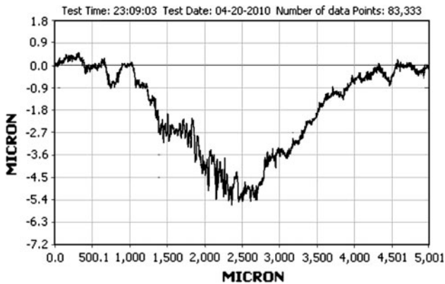
Fig. 7 Wear track produced on counter material (EN32) after CrAlN-coated pin slide over specific time period (test condition: 10 N, 0.5 m/s, 2000 m sliding distance, 30 °C, 32%Rh)
